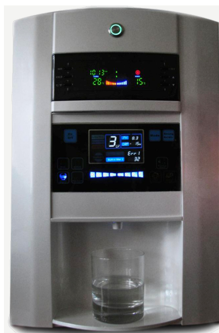
Figure 1: Device "WaterLife" that produces water with plus and minus redox potential.
